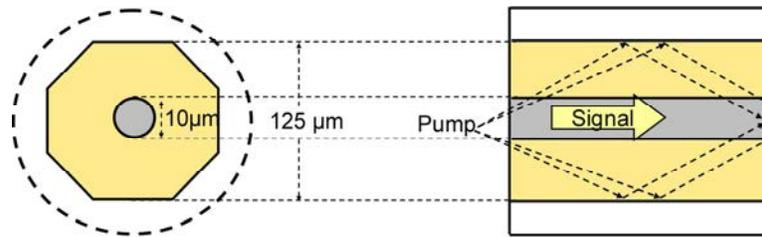
Fig. 1. Geometry of the EYDF.
