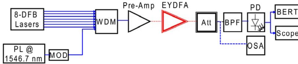
Fig. 6. Gain, NF and Bit error ratio measurement setup. PL: Probe Laser, Mod: Modulator, WDM: Wavelength Division Multiplexer, Att: variable Attenuator, BPF: Bandpass filter @ 1546.7 nm, PD: Photodiode, OSA: Optical Spectrum Analyzer, BERT: BER Tester.
