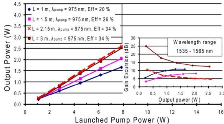
Fig. 4. Total output power versus launched pump power for different lengths of EYDF. Inset: Gain excursion over the wavelength range of 1535-1565 nm versus the total output power.
