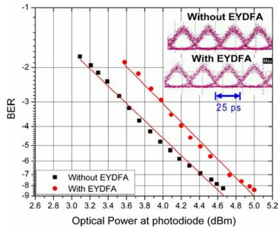
Fig. 9. Bit error ratio and eye diagrams at 40 Gb/s with and without the EYDFA in the communication link.
