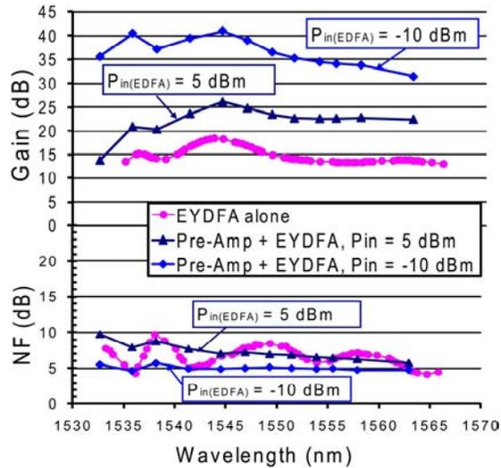
Fig. 8. Gain and noise-figure (NF) of the EYDFA as well as that of the pre-amplifier followed by the EYDFA at different amounts of power at the input of the preamplifier
