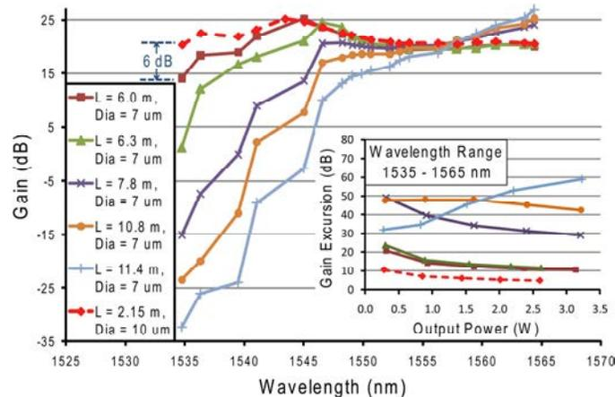
Fig. 5. Gain spectrum for different lengths of single-mode EYDF (core diameter =  $7 \mu\text{m}$ ) and for 2.15 m of multimode EYDF delivering a total output power of  $\sim 33.9$  dBm. Inset: Gain excursion over the wavelength range of 1535-1565 nm versus the total output power.
