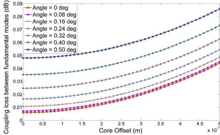
Fig. 2. Bit Coupling loss between guided mode of single-mode fiber and the fundamental mode of EYDF versus the lateral misalignment in terms of core offset for different angular misalignment values.
