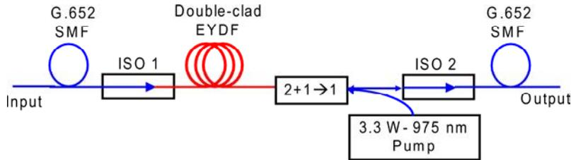
Fig. 3. Schematic of the EYDFA. ISO: Isolator, SMF: Single Mode Fiber.
