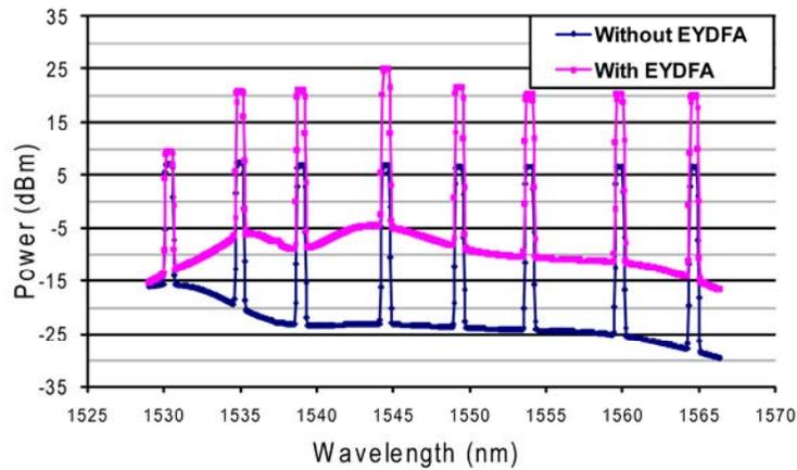
Fig. 7. Spectra before and after amplification of 8 channels spreading from 1530.3 nm to 1564.8 nm.
